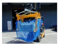
also attached to each side/pivot hook, which will remove any slack in the net, ensuring should the load fail the contents will be caught by the net. The net must enclosed the four legs as shown in photo. If in any doubt about usage of the safety net with Block Grab in a particular situation, consult the site Health & Safety Officer.
