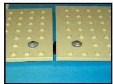
Step 4: Place second bolt and washer into fixture and Hand tighten bolt .
