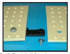
Step 3: Place bolt with flat washer into fixture with imbeded nut.
