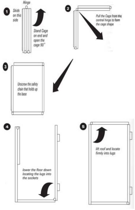
**To Dismantle:** open door. Lift Base and secure using the safety chain. Lower the roof. From inside unit, pull back left corner towards you, and concertina other 2 sides. Push the door to the base and lower unit onto the skids.
