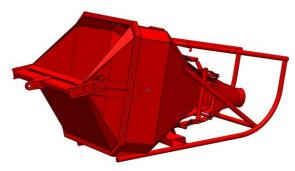
Column Skips are designed to allow concrete to be poured into columns or shuttering with narrow or difficult access and discharged at low level, reducing the risk of aggregate separation.
