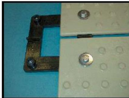
Step 3: Slide second mat on to fixture and install bolt.
